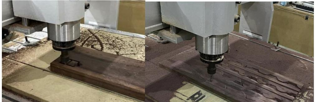
Gambar 5. 8 Proses *CNC interlocking joining*
