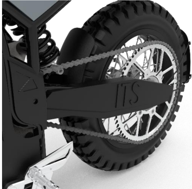
Gambar 4 6 Desain cover swing arm
