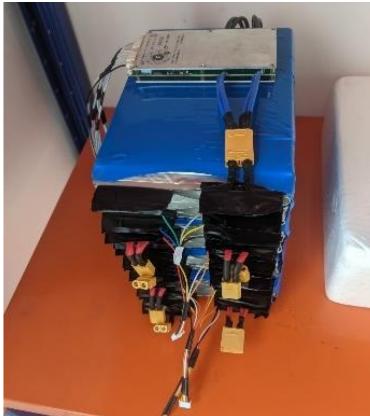
Gambar 4.13 Battery pack LiFePO4 3.8KwH dan BMS
