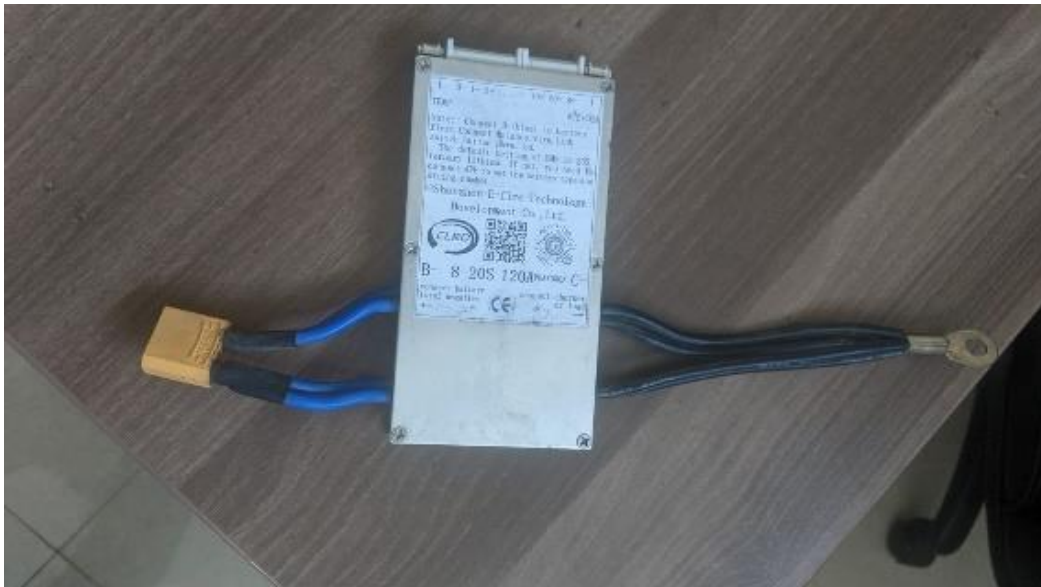
Gambar 4 28 Battery Management System
