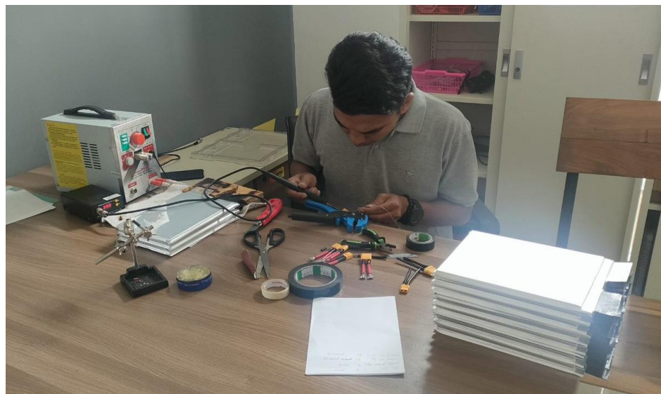
Gambar 4 20 proses fabrikasi battery pack
