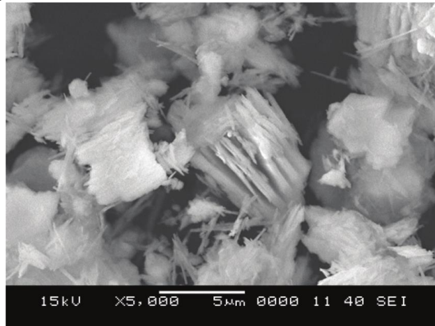
Gambar 2.5 Morfologi Metakaolin (800°C selama 2 jam) hasil uji SEM (Abdullah et al., 2018)
