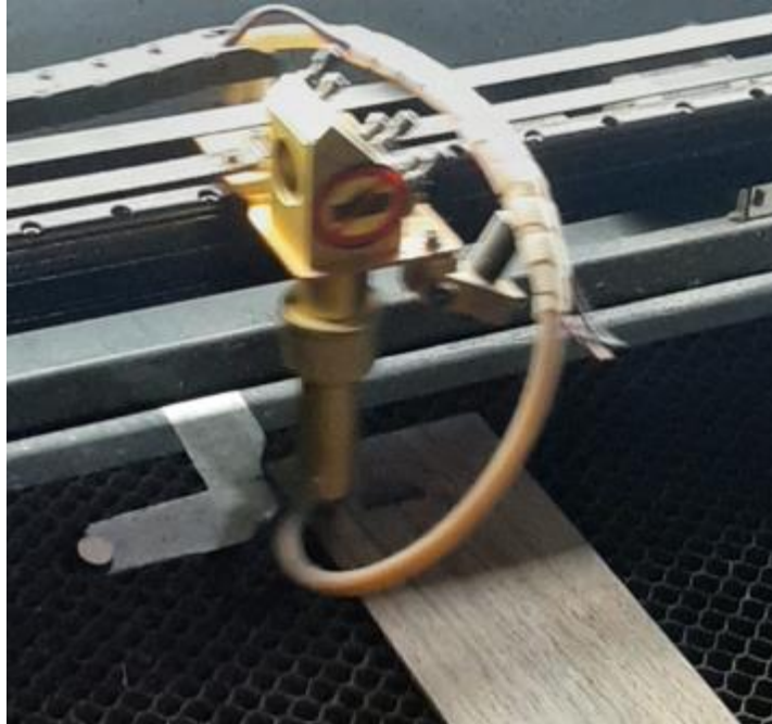
Gambar 5.23 Proses laser cutting backcase ( sumber: Olahan Pribadi)
