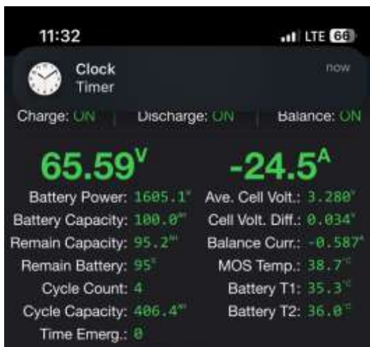
Figure 5.21 Battery Capacity for 24 Ampere in Pitch 8 Propeller After Running
