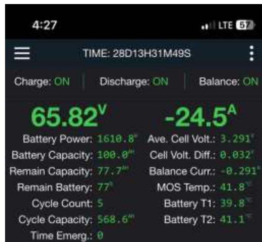
Figure 4.7 Battery Capacity for 24 Ampere in Pitch 12 Propeller Before Running
