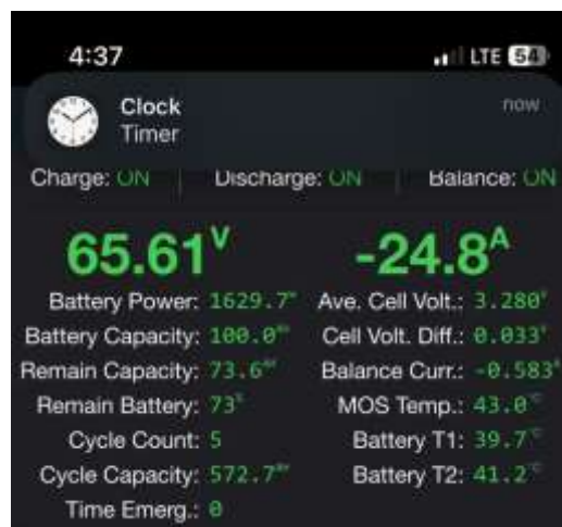
Figure 4.8 Battery Capacity for 24 Ampere in Pitch 12 Propeller After Running
