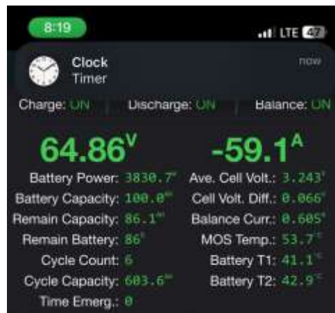
Figure 4.10 Battery Capacity for 60 Ampere in Pitch 12 Propeller After Running
