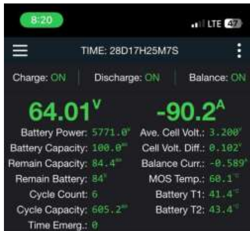
Figure 4.11 Battery Capacity for 90 Ampere in Pitch 12 Propeller Before Running
