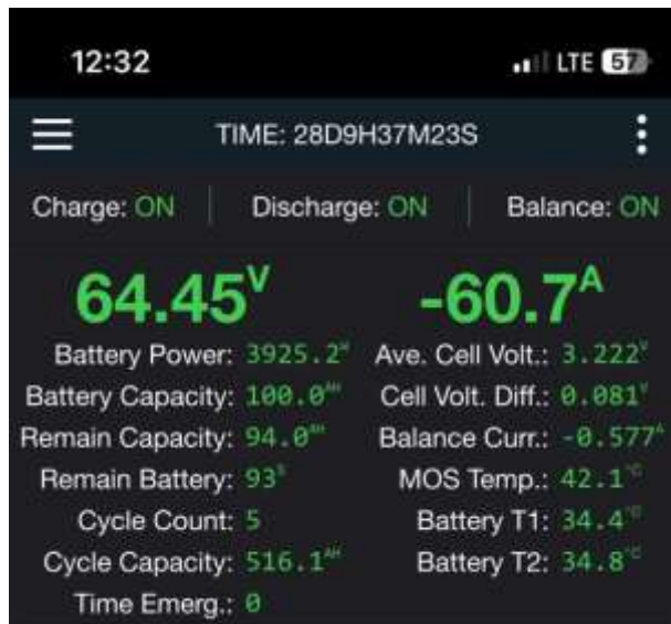
Figure 5.28 Battery Capacity for 60 Ampere in Pitch 9 Propeller Before Running
