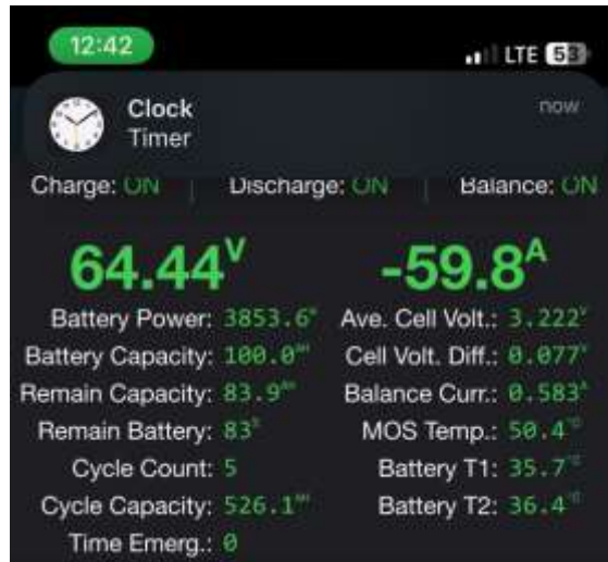
Figure 5.29 Battery Capacity for 60 Ampere in Pitch 9 Propeller After Running
