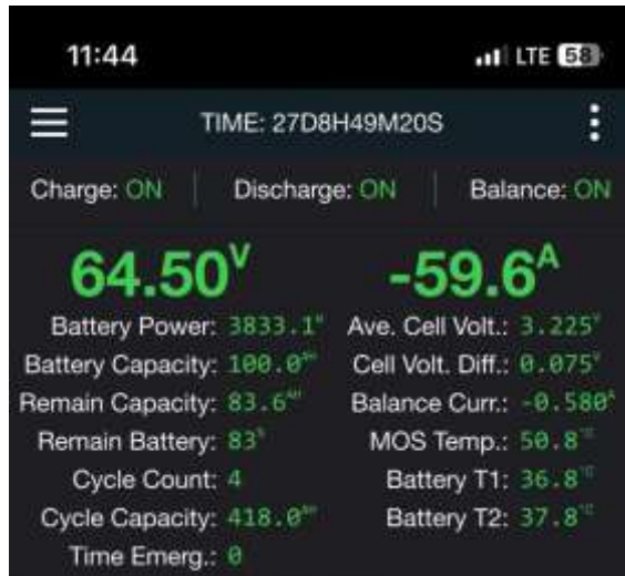
Figure 5.23 Battery Capacity for 60 Ampere in Pitch 8 Propeller After Running
