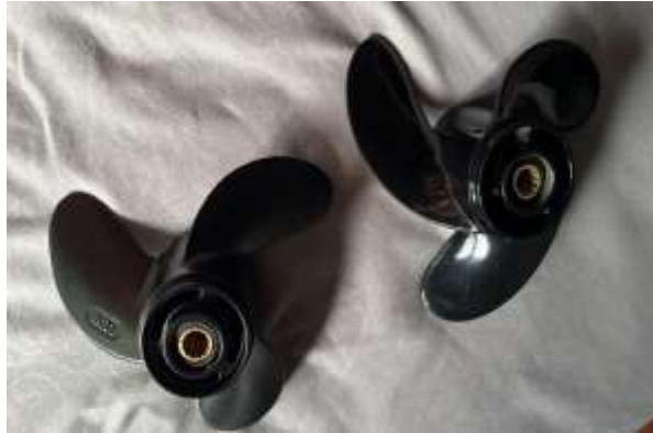
Figure 3.3 Propeller Variation 7,8 x 8 ; 7,8 x 9; and 7,8 x 12 (Personal Documentation)
