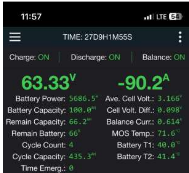
Figure 5.25 Battery Capacity for 60 Ampere in Pitch 8 Propeller After Running
