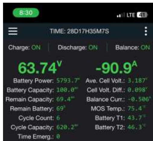
Figure 4.12 Battery Capacity for 90 Ampere in Pitch 12 Propeller After Running
