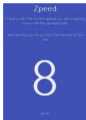
Figure 5.16 Speed to arrive of Boat that used Electric Outboard with Propeller Pitch 8 in 60 Ampere of current input (Personal Documentation)
