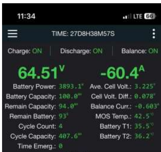
Figure 5.22 Battery Capacity for 60 Ampere in Pitch 8 Propeller Before Running
