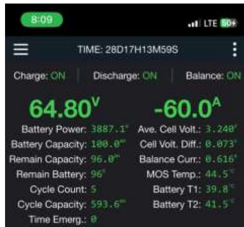
Figure 4.9 Battery Capacity for 60 Ampere in Pitch 12 Propeller before Running
