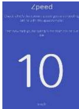
Figure 4.3 Speed to Depart of Boat that used Electric Outboard with Propeller Pitch 9 in 60 Ampere of current input (Personal Documentation)
