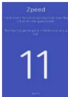
Figure 4.16 Speed to Depart of Boat that used Electric Outboard with Propeller Pitch 9 in 90 Ampere of current input (Personal Documentation)
