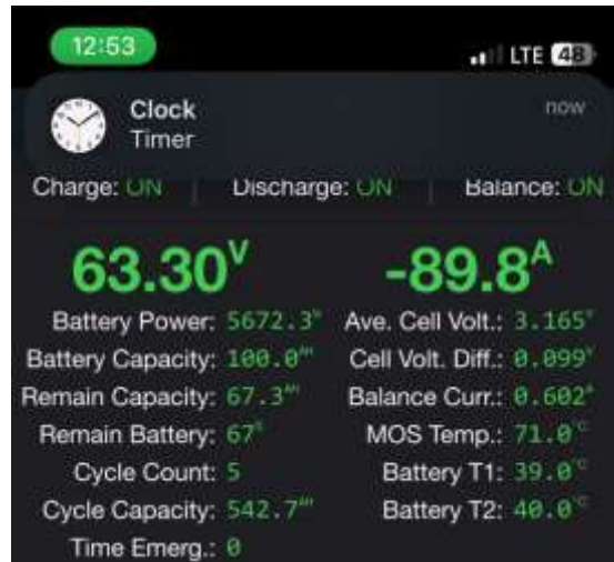
Figure 5.31 Battery Capacity for 90 Ampere in Pitch 9 Propeller After Running
