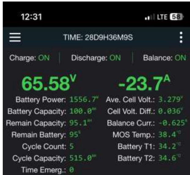
Figure 5.27 Battery Capacity for 24 Ampere in Pitch 9 Propeller After Running
