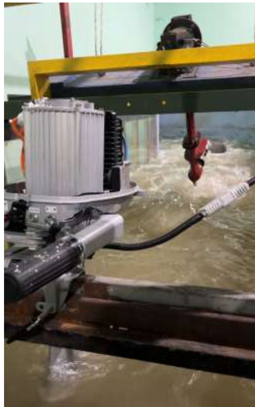
Figure 3.5 Cerano Electric Outboard Running to Getting Energy Consumption (Personal Documentation)
