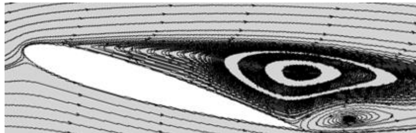
Gambar 4. 6 Streamline Airfoil Polos Saat Angle of attack 16^\circ .
