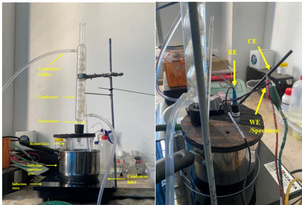
Gambar 3. 15 Instalasi Pengujian Potentiodynamic Polarization
