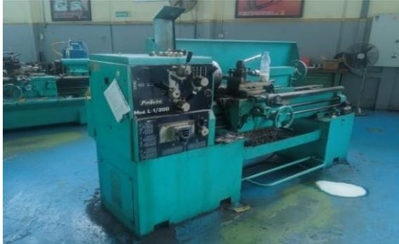
**Gambar 2. 9** *Conventional lathe machine Pinacho Mod.L-1/200*
