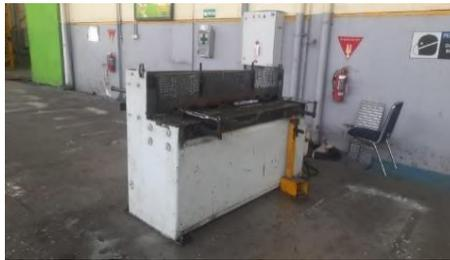
**Gambar 2. 30** Mesin *Shearink* Fintech P-0010
