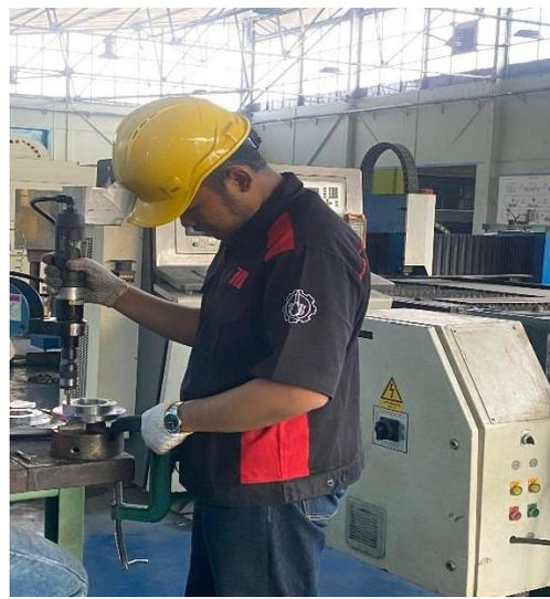
Mengoperasikan *Hydraulic Tapping Machine*
