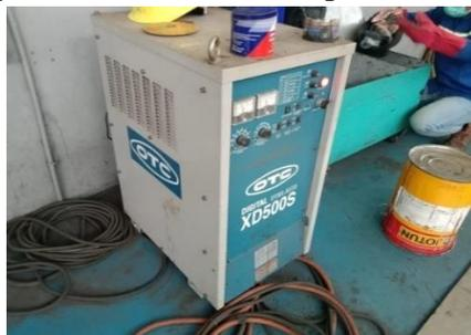
**Gambar 2. 21** Mesin Las Digital Dyna Auto CO2/MAG tipe CPXD-500SII (GMAW)
