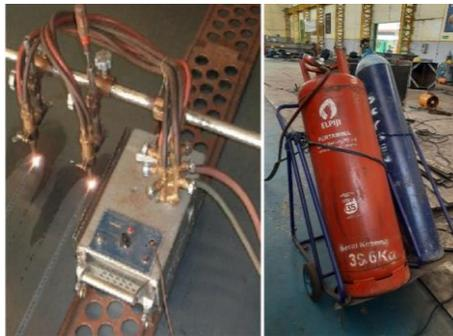
**Gambar 2. 25** Gas Metal Cutting type CGI-30
