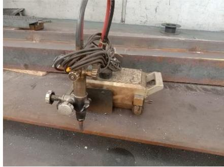
**Gambar 2. 26** Gas Metal Cutting type KC-12 Mini
