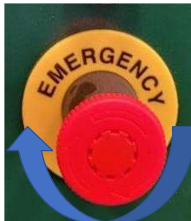
Gambar 4.19 Release tombol Emergency Stop (sumber : PT. Matahari Megah)
