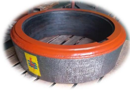
**Gambar 2. 13** Grinding Tyre Pulverizer Coal Mill
