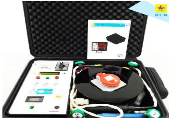
**Gambar 2. 16** Portable Change Over Switch
