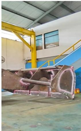
**Gambar 4. 10** Proses Developer dan Cleaning
