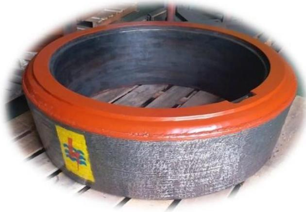
**Gambar 2. 11** Grinding Tyre Pulverizer Coal Mill
