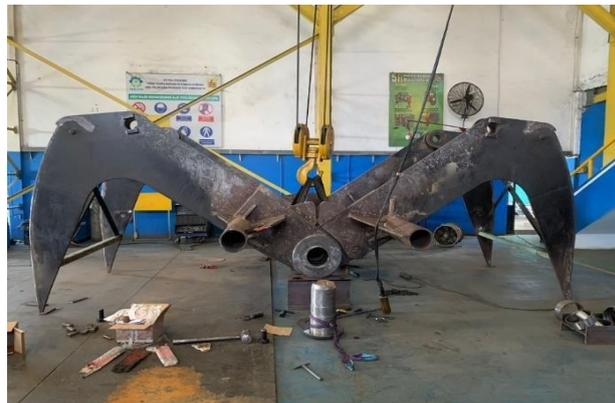
**Gambar 4. 13** Proses Assembly Scoop Assy
