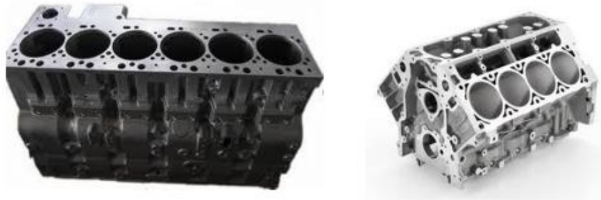
Gambar 4.35 Cylinder Block Engine Inline Type dan V Type (Sumber : Basic Mechanic Course, 2011 )
