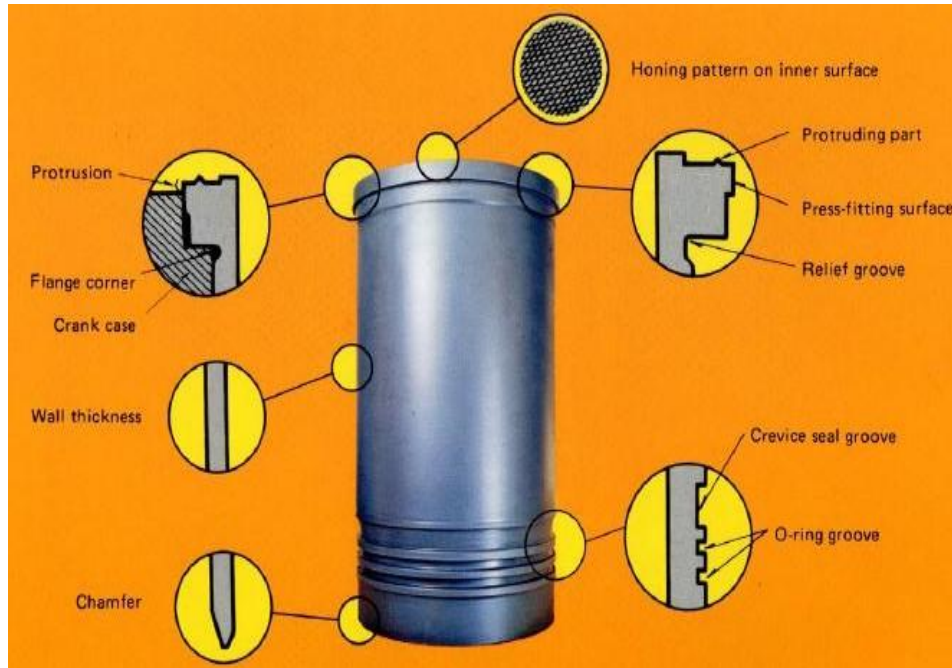
Gambar 4.39 Struktur Liner (Sumber : Basic Mechanic Course, 2011)
