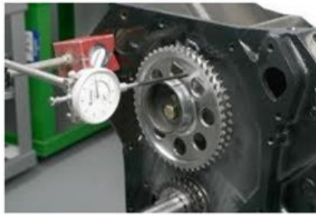
Gambar 4.74 Pengukuran Timing Gear (Sumber : Basic Mechanic Course , 2011)
