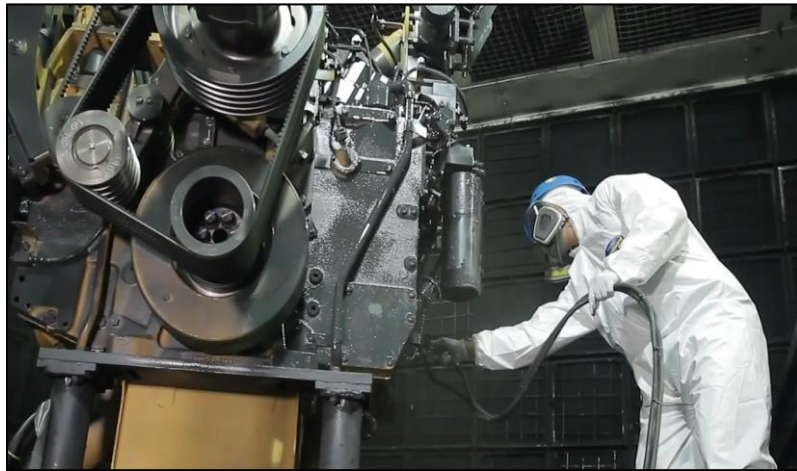
Gambar 2.16 Proses Pinting (Sumber : PT. Komatsu Remanufacturing Asia)
