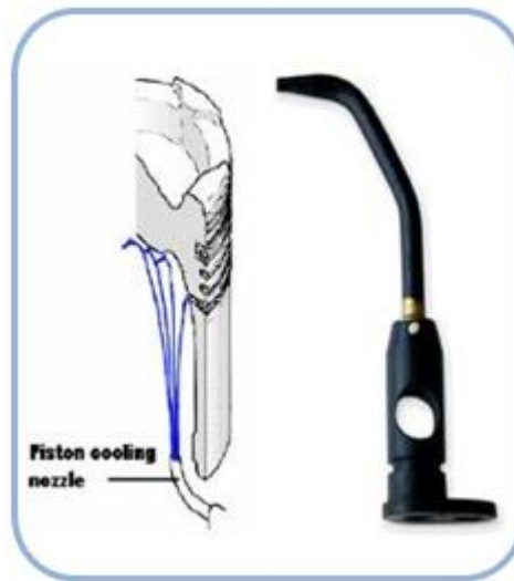
Gambar 4.48 Piston Cooling Nozzle (Sumber : Basic Mechanic Course, 2011 )
