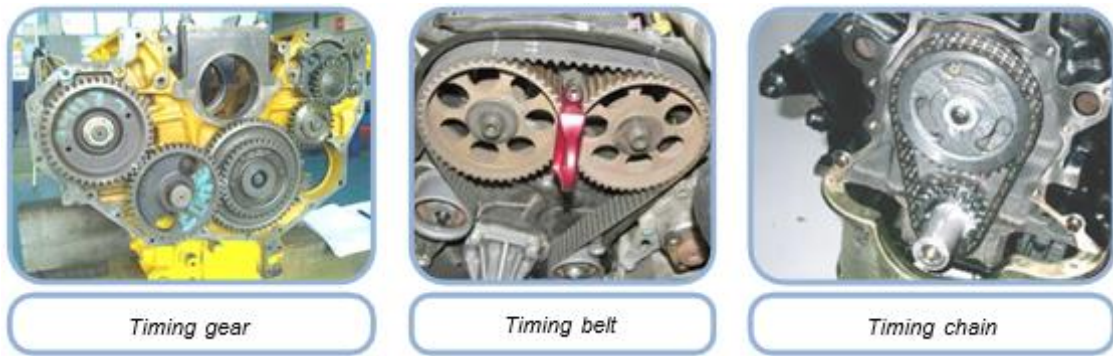
Gambar 4.57 Contoh Timing Gear , Timing Belt , Timing Chain (Sumber : Basic Mechanic Course , 2011)
