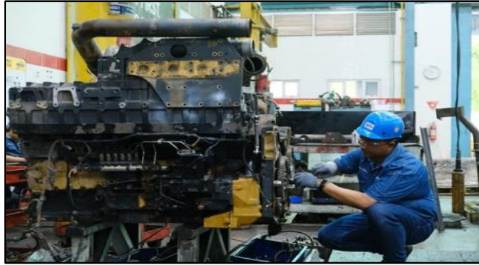
Gambar 2.11 Proses disassembly (Sumber : PT. Komatsu Remanufacturing Asia)
