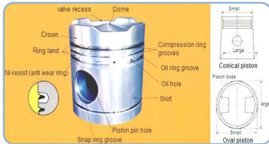
Gambar 4.47 Struktur Piston (Sumber : Basic Mechanic Course, 2011 )
