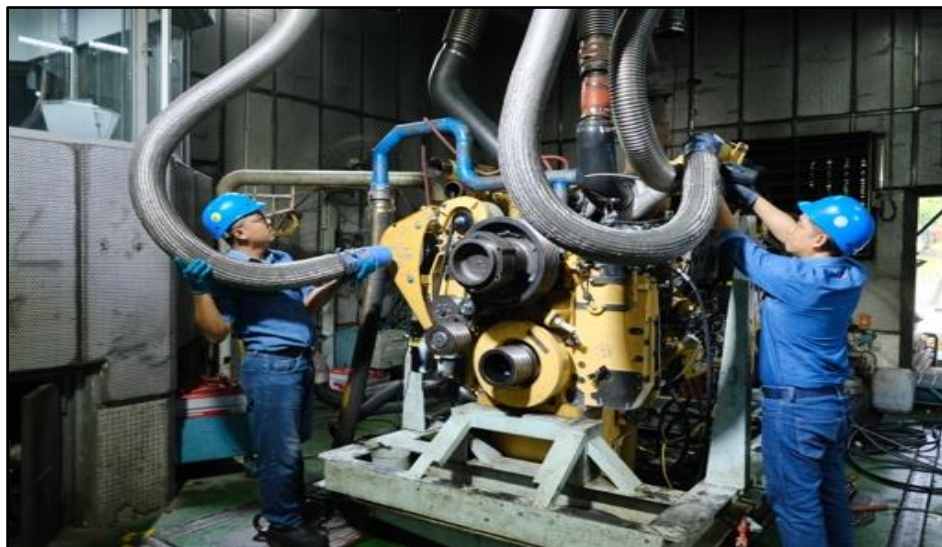
Gambar 2.15 Proses Performa Test (Sumber : PT. Komatsu Remanufacturing Asia)
