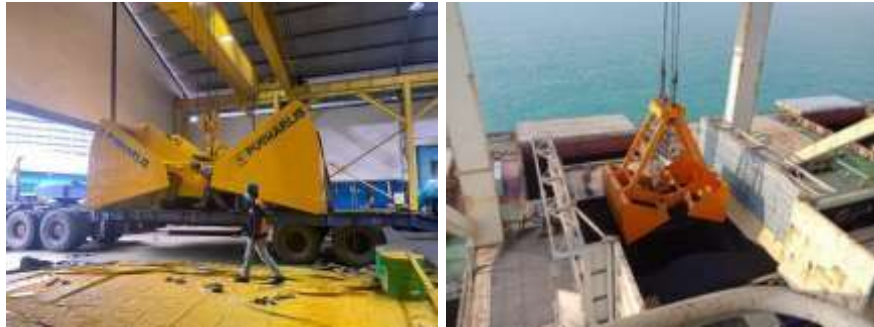
Gambar 2. 11 Grab Ship Unloader & Accessories
