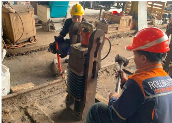
**Gambar 3.11** *Assembly Draft Gear*
