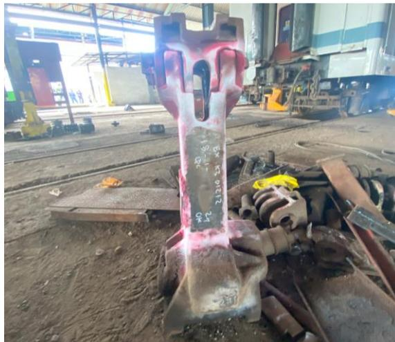
**Gambar 3.8** Liquid Penetrant Test Pada Coupler
