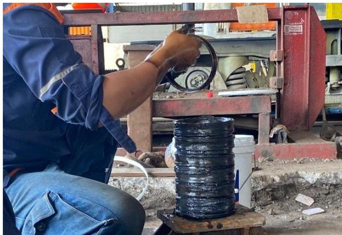
**Gambar 3.15** Menyusun Pegas *Draft Gear* Tabung
