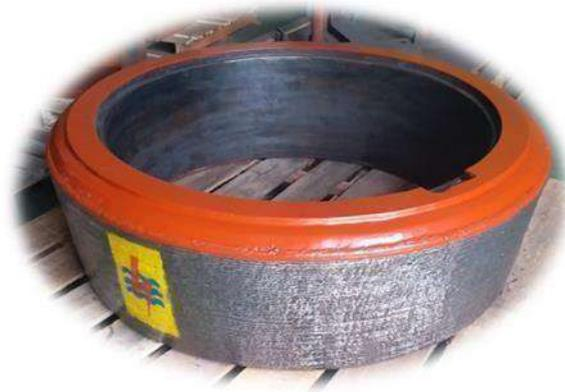
**Gambar 2.11** Grinding Tyre Pulverize Coal Mill
