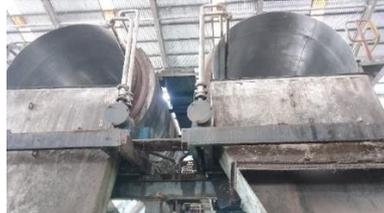
**Gambar 3. 20** Rotary Vacuum Filter
