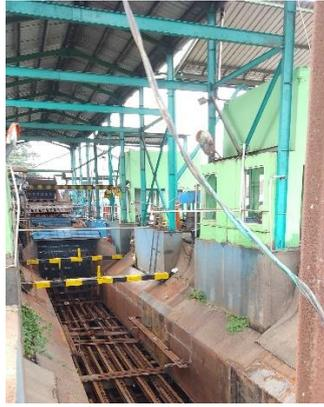
**Gambar 3. 6** Auxiliary Cane Carrier
