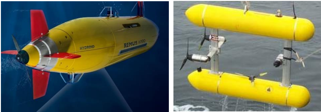
Gambar 1. 1 AUV Single-body (Keller, 2016) dan Multi-body (Ferrini, Singh, Clarke, Wakefield, & K., 2006)
