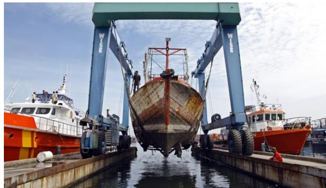
Gambar 2. 6 Marine Travel Lifts
