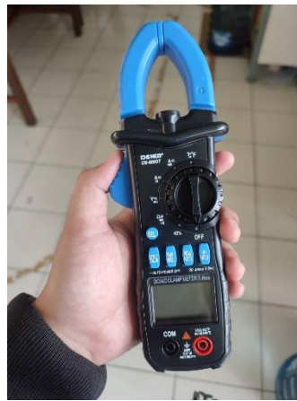
Gambar A.9 Clampmeter
