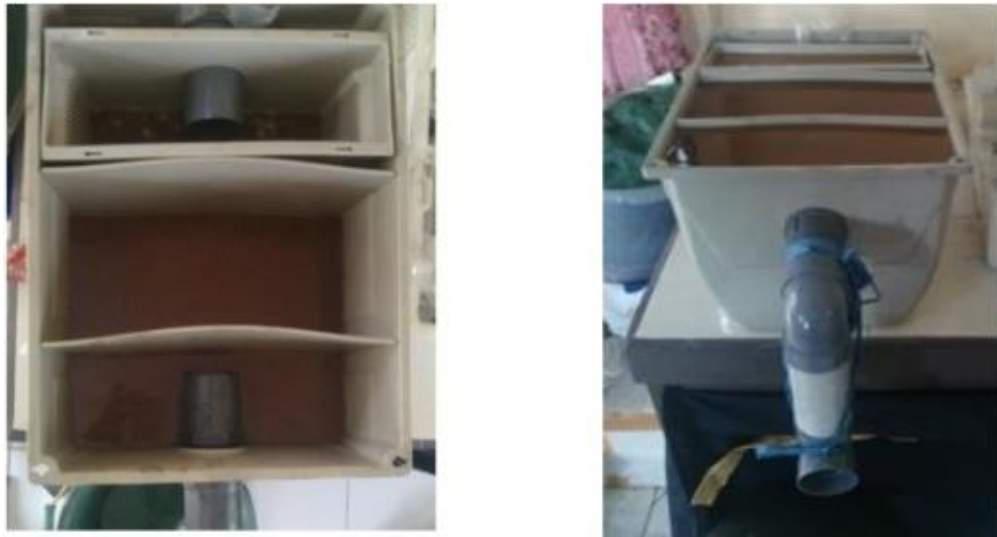
Gambar 4. 10 Grease Trap Sumber : Zahara dkk, 2017
