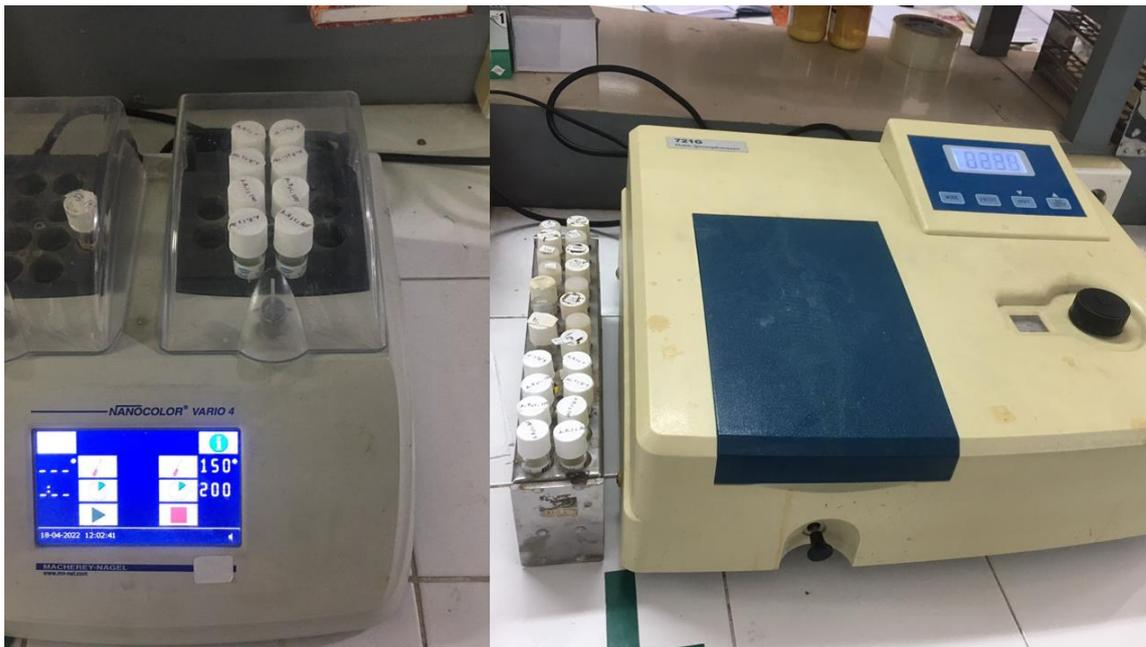
Gambar F. 6 Analisis COD Metode *Closed Reflux*
