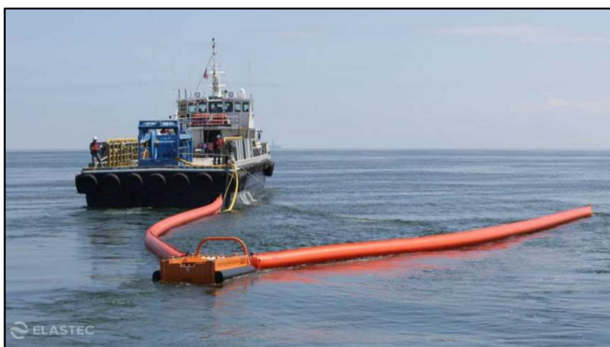
Gambar 4.15 Penggunaan oil boom dan oil skimmer Sumber: elastec.com/one-skimmer-released (2015)
