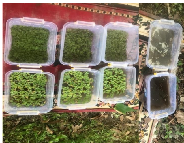
Gambar 4.12 Reaktor Uji Fitotreatment
