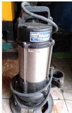
Gambar 4. 1 Pompa Submersible HCP Pump
