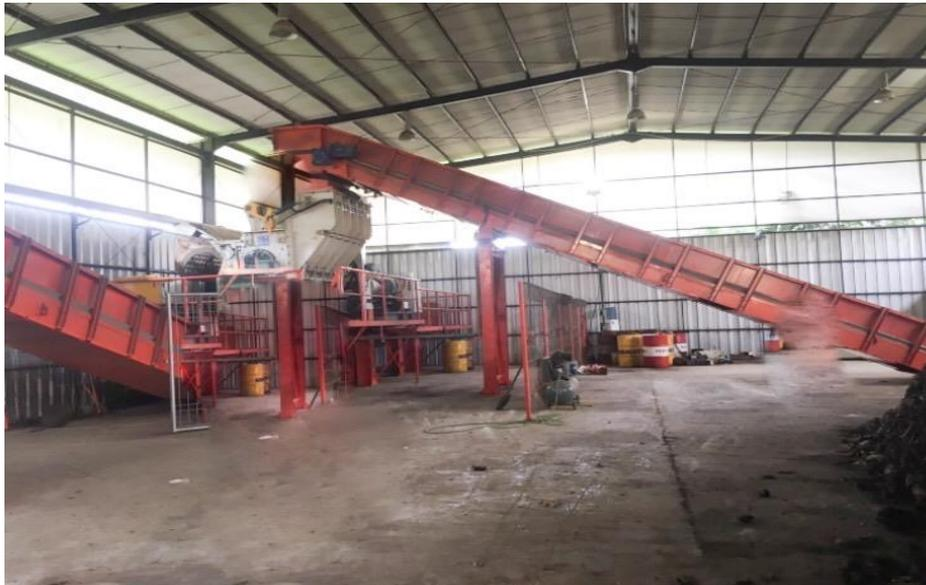
**Gambar 4.9 *Fine Shredder***
