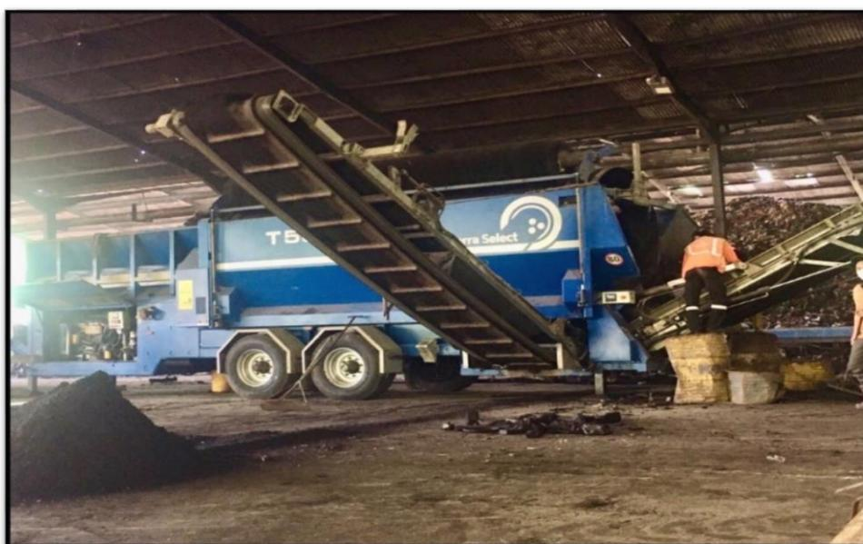
**Gambar 4.8 *Trommel Screen Berukuran 10 mm***
