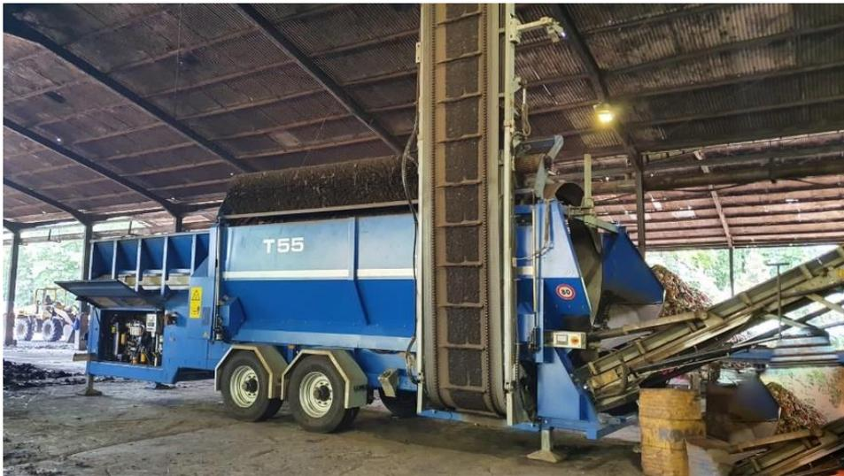
**Gambar 4. 5 *Trommel Screen* Berukuran 30 mm**
