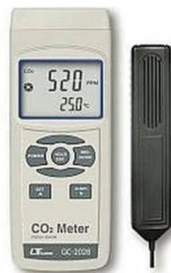
Gambar 3. 1 CO<sub>2</sub> Meter Tipe Lutron GC-2028
