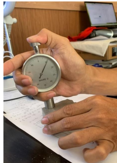
Gambar Hasil Uji Hardness PU+Nano0%+Bam 10%
