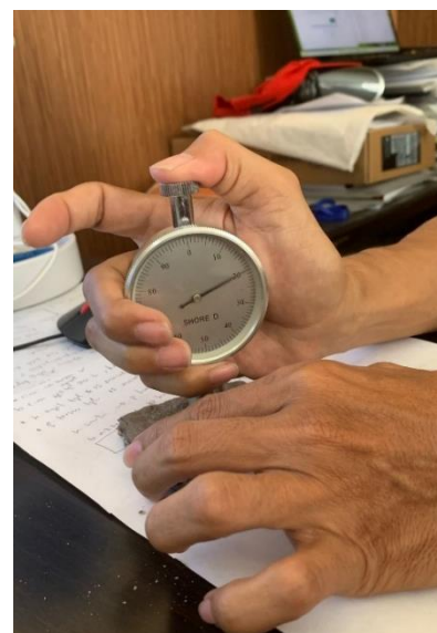
Gambar Hasil Uji Hardness PU+ Nano 15%+Bam 10%
