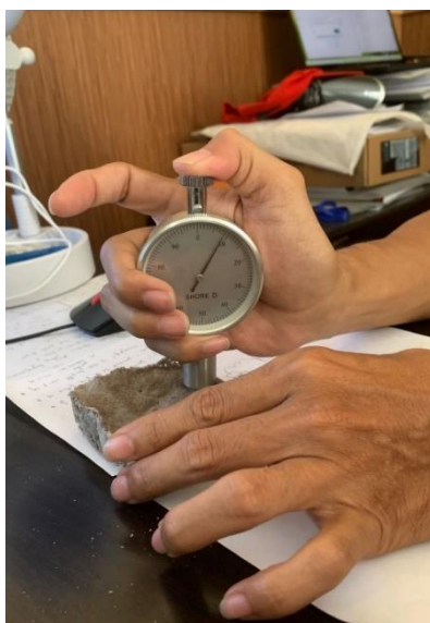
Gambar Hasil Uji Hardness PU+ Nano 10%+Bam 10%
