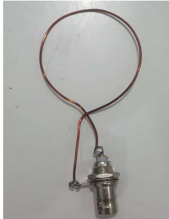
**Gambar 3. 8** Desain *Loop Antenna* (Bestowan, 2019)
