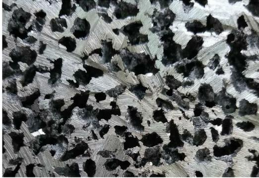
**Gambar 4.1** Hasil pengecoran aluminium *foam*
