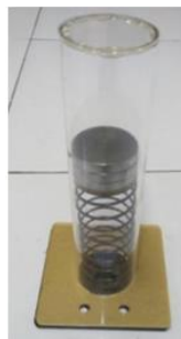
Gambar 2.19 Translational Mass Vibration Absorber (TMVA) (Lestari, 2019)
