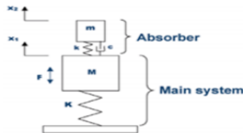
Gambar 2.17 Model Dinamis Simulasi 2 DoF damped DVA (Pachpute, 2016)
