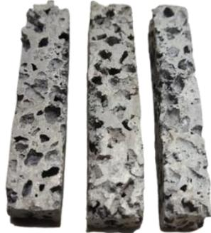
**Gambar 4.10** Spesimen uji impak paduan Al-Mg-Si foam
