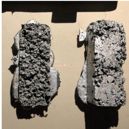
Spesimen aluminium *foam* hasil pengecoran (gagal)
