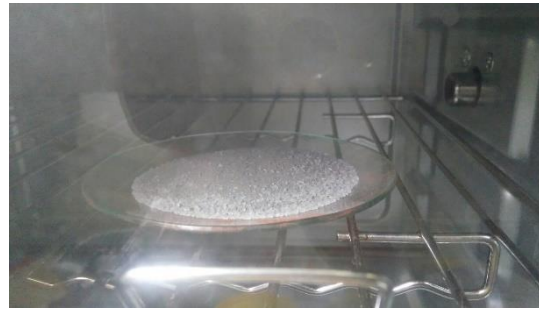
Gambar 3.13 Proses drying serbuk PA6
