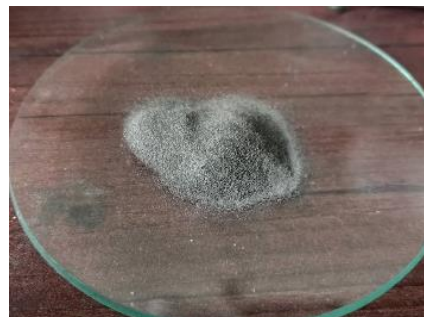
Gambar 3. 10 Serbuk Stainless Steel 304L
