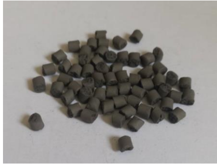
Gambar 2.12 Feedstock injection molding
