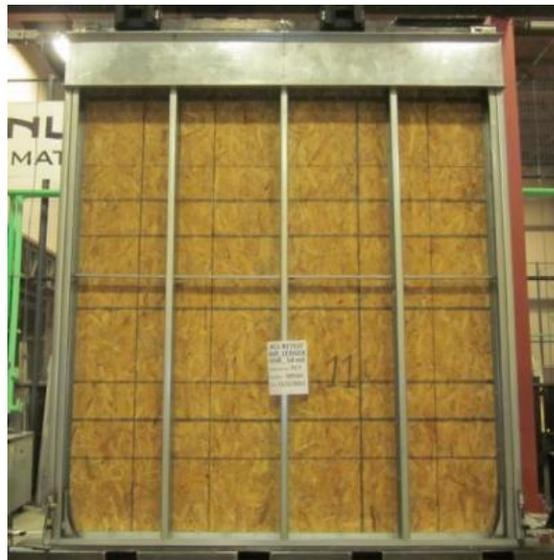
Gambar 2.1 CFS *light-frame shear walls sheathed with wood structural panels* (Liu, Peterman and Schafer, 2014)
