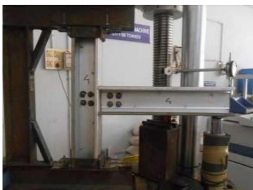
Gambar 2.4 *CFS special bolted moment frames* (Kaling dkk., 2015)
