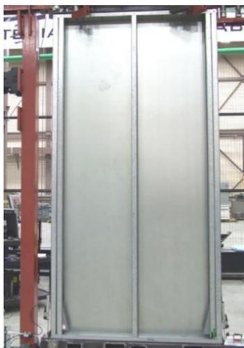
Gambar 2.2 *CFS light-frame shear walls sheathed with steel sheet sheathing* (Yu, 2010)
