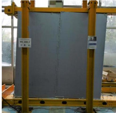
Gambar 2.5 *CFS light-frame shear walls sheathed with gypsum board* (Macillo dkk., 2017)
