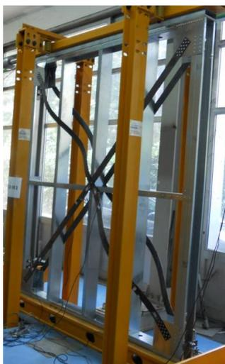
Gambar 2.3 *CFS light-frame strap-braced wall systems* (Fiorino dkk., 2016)
