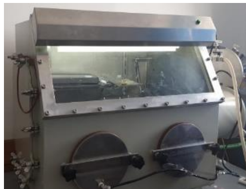
Gambar 3. 26 Glove Box Laboratorium Korosi
