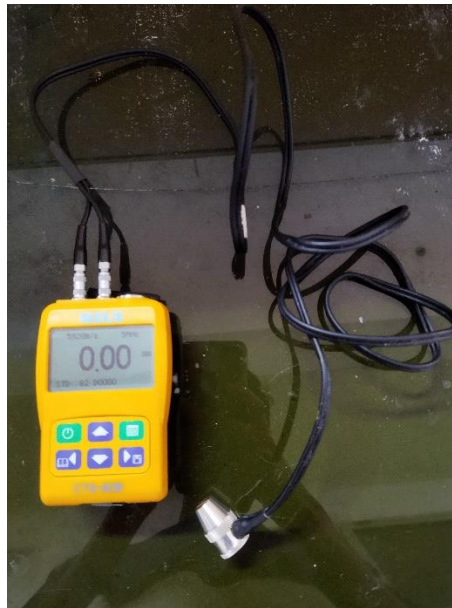
Gambar 3.16 Ultrasonic Thickness Gauge SIUI CTS 30B
