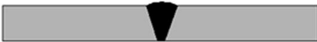
Gambar 2. 6 Contoh Butt Joint (Utomo, 2019)
