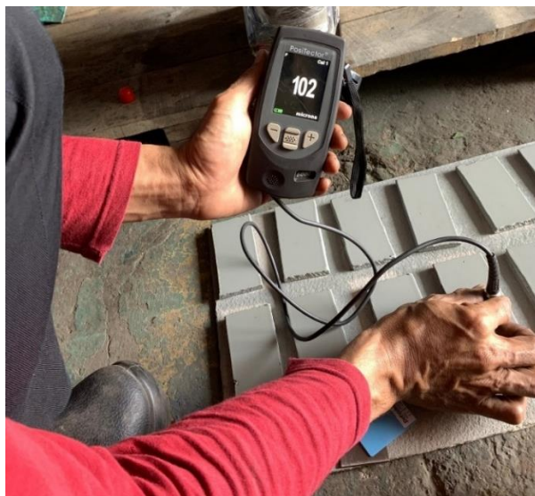
Gambar 3.20 Pengukuran Dry Film Thickness (DFT)
