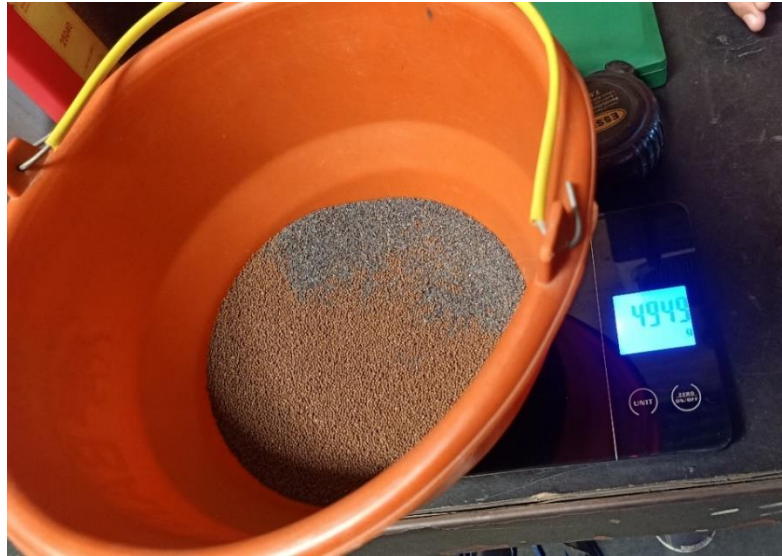
Gambar 3.9 Pencampuran Material Abrasif ( Steel Grit 45 : Steel Shot 20 : Bekas 30 )
