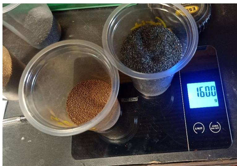
Gambar 3.8 Pencampuran Material Abrasif ( Steel Grit 60 : Steel Shot 40)
