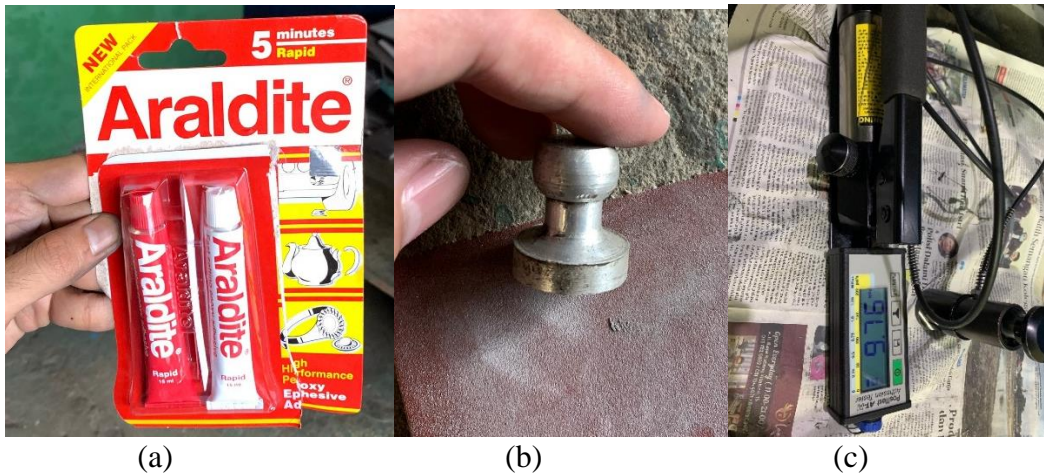
Gambar 3.21 (a) Lem Epoxy Araldite, (b) Dolly 20mm, (c) Portable Adhesion Tester
