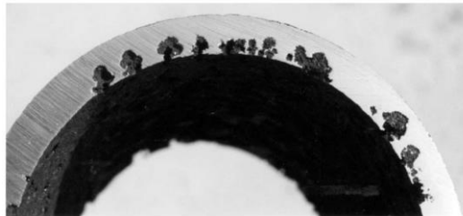
Gambar 2.7 Pitting Corrosion (Davis, 2000)
