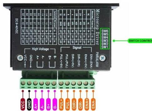
Gambar 2. 9 Driver Motor Stepper TB6600
