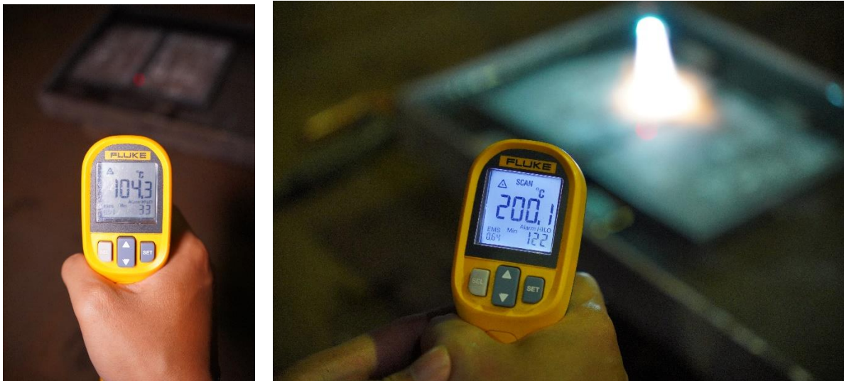
Gambar 3. 2 Pengukuran Preheating Temperature
