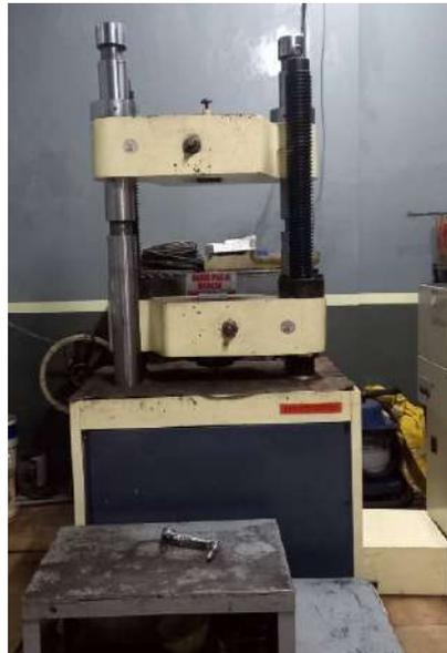
Gambar 3. 11. HT-950 Universal Testing Machine
