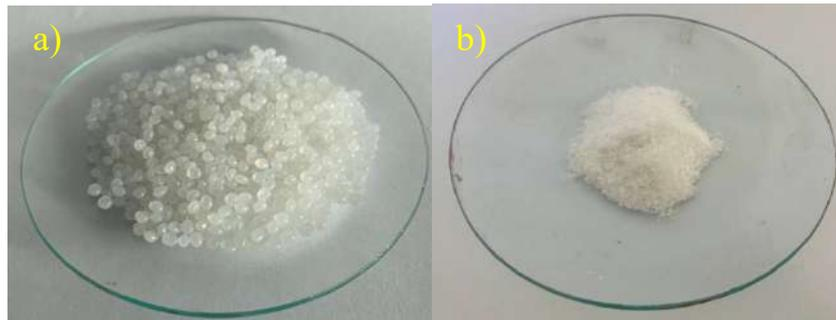
Gambar 4. 4. Poliamida 6 (a) Sebelum *grinding* (b) Sesudah *grinding*
