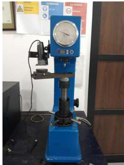
Gambar 3. 9. *Hardness testing machine*
