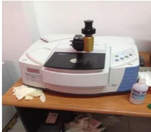
**Gambar 3.5** Instrumen FTIR
