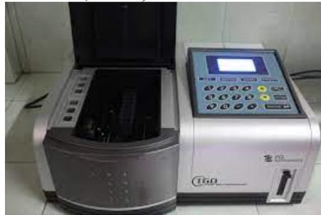
**Gambar 3. 11** Instrumen UV Vis
