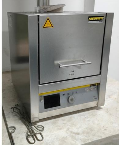
Gambar 3. 9 Alat uji *Volatile Matter*
