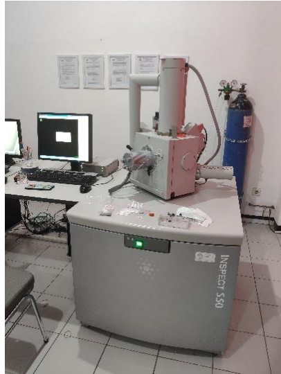
Gambar 3.16 Alat uji SEM-EDX FEI Tipe Inspect S-50
