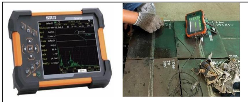
Gambar 3.5 Alat Uji Ultrasonik
