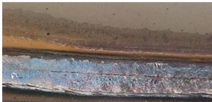
**Gambar 2.11** Skema *Hot Cracking*
