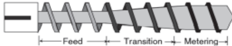
Gambar 2.9 Extruder Screw (Giles et al., 2005)
