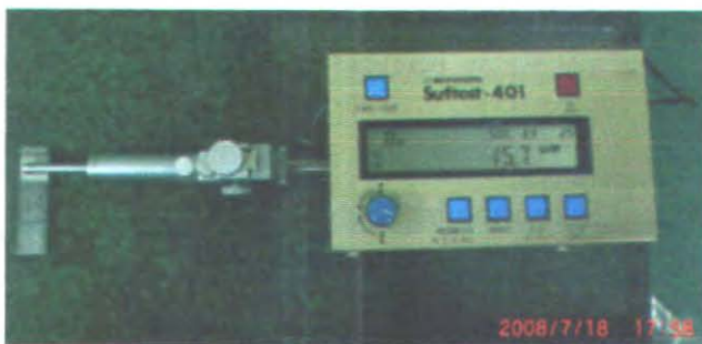
Gambar 3.6 Surface roughness tester (MITUTOYO SurfTest-401 )
