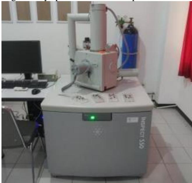
**Gambar 3.5** Alat uji SEM-EDX Inspect S-50
