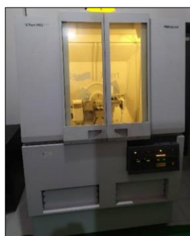
Gambar 3.5 Alat Pengujian X-Ray Diffractometer (XRD) Testing
