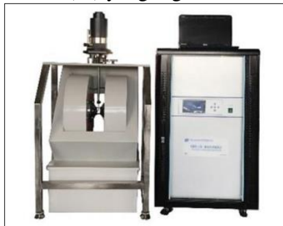
Gambar 3.9 Alat Pengujian Vibrating Sample Magnetometer (VSM) Testing
