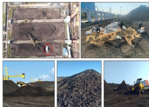
Gambar 3.5 Proses Blending Batubara dan Sekam Padi di Coal Yard
