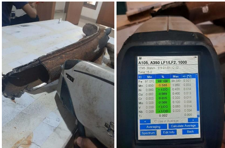
Gambar 4.9 Lokasi pengujian Positive Material Identification Bruker S1 Titan
