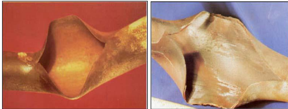
Gambar 2.8 Kegagalan short term overheating [18]
