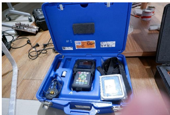
Gambar 3.5 Ultrasonic Thickness Gauging Olympus
