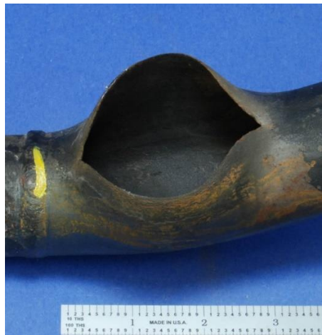
Gambar 2. 19. Kegagalan short term overheating
